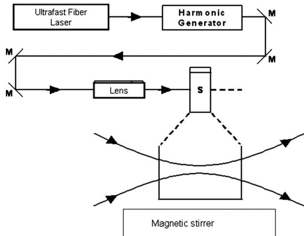
**Fig. 1** Experimental setup for the inactivation of viral particles with a near-IR subpicosecond fiber laser: M, mirror; S, vial containing viruses in buffer solutions.
