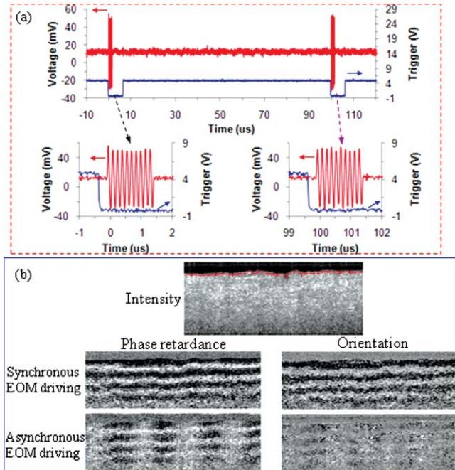
**Fig. 1** (a) Example of the generated synchronized 10-cycle sinusoidal waveform using the A-trigger signal from the swept source as an external trigger source by using the triggered tone-burst mode of the function generator. (b) Measured phase retardance and orientation images on the same equine tendon sample by using asynchronous and synchronous EOM driving.
