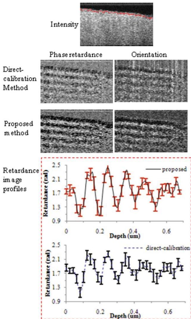
**Fig. 2** Measured phase retardance and orientation images of equine tendon by using the proposed method and the direct-calibration method of determining the surface Jones matrix, respectively. Profiles of images are also included, together with the variance about the mean.
