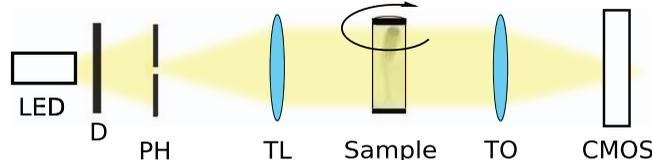
**Fig. 1** Scheme of the experimental setup for flow-OPT (D: diffuser; PH: pinhole; TL: telecentric illumination lens, TO: telecentric objective.)
