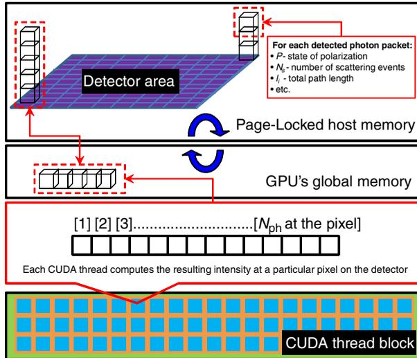
**Fig. 3** The block-diagram presents the principles of O3MC GPU-based computations of the resulting intensity of scattered light and its spatial distribution at the detector area. Each pixel at the detection area is associated with  $(x, y)$  coordinates and contains  $N_{ph}$  photon trajectories.
