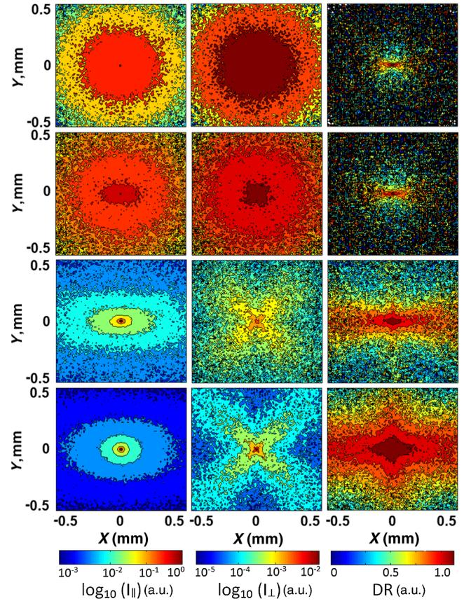
**Fig. 6** Surface distributions of  $I_{\parallel}$ ,  $I_{\perp}$ , and depolarization ratios of backscattered linearly polarized light for various values of scattering anisotropy: from the top  $g = 0, 0.5, 0.9$  and  $0.98$ . MC simulations were performed with noncoherent light ( $l_c = 0$  mm) normally incident on the semi-infinite scattering medium with  $\mu_s = 30 \text{ mm}^{-1}$ ,  $\mu_a = 0.001 \text{ mm}^{-1}$ , and detected over entire medium surface.
