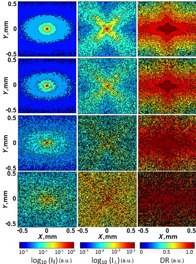
**Fig. 8** Intensity distributions of  $I_{\parallel,\perp}$  and the depolarization ratios DR at the surface of the medium for backscattered linearly polarized light of various coherence lengths  $l_c$ , from top:  $l_c = 0.01 \mu\text{m}$ , 0.1 mm, 1 mm, 1 m, counted for a highly anisotropic scattering medium with  $g = 0.98$ ,  $\mu_s = 30 \text{ mm}^{-1}$ ,  $\mu_a = 0.001 \text{ mm}^{-1}$ .
