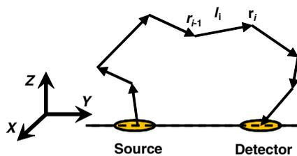
**Fig. 2** Stochastic trajectory of a photon packet traveling from the point of incidence (source) to the point of detection (detector);  $\mathbf{r}_{i-1}$  and  $\mathbf{r}_i$  are the  $i-1$  and the  $i$  scattering events, and  $l$  is the photon packet's pathlength at the  $i-1$  scattering event.
