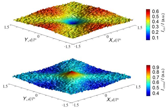
**Fig. 9** Surface distributions of  $I_{\text{co}}$  (top) and  $I_{\text{cross}}$  (bottom) polarized components of backscattered circularly polarized light,  $d$  is the distance at the surface,  $l^* = 1/\mu_s^*$ ; counted for a semi-infinite scattering medium ( $\mu_s = 30 \text{ mm}^{-1}$ ,  $\mu_a = 0.001 \text{ mm}^{-1}$ ,  $g = 0.98$ , and  $n = 1.5$ ).
