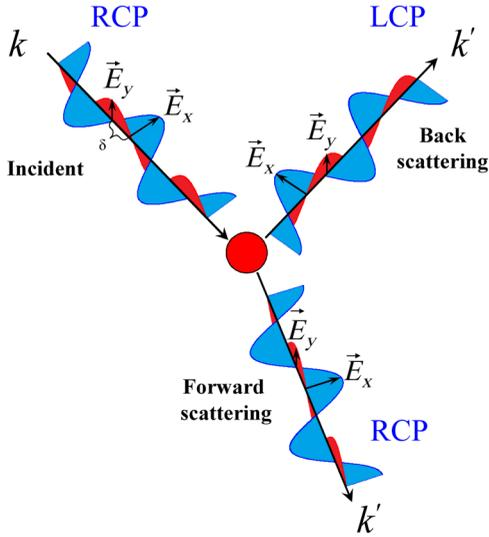
**Fig. 5** Schematic presentation of forward and backscattering for circularly polarized light. When right-handed circular polarization (RCP) light is scattered in forward direction ( $\widehat{kk}' < \pi/2$ ) its helicity is preserved, whereas for backscattered light ( $\widehat{kk}' > \pi/2$ ), the phase shift  $\delta = \phi_x - \phi_y$  between  $E_x$  and  $E_y$  is reversed, causing the light to change from RCP to left-handed circular polarization (LCP).
