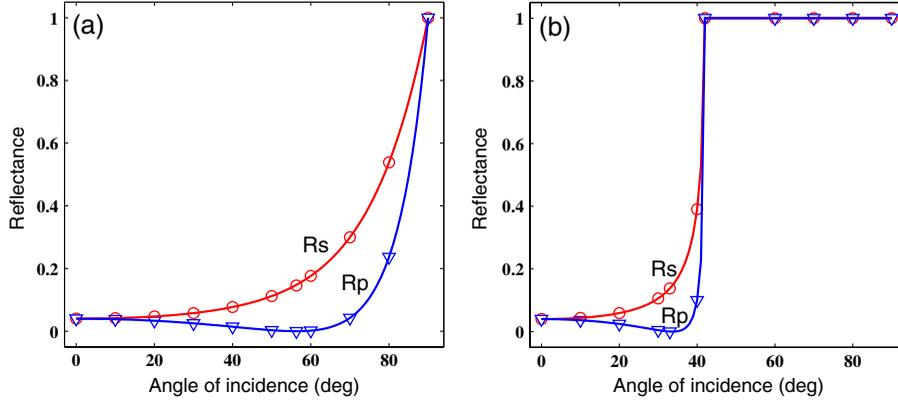
**Fig. 4** Fresnel reflection coefficients  $R_s$  (circles) and  $R_p$  (triangles) for light traveling: (a) from air ( $n_1 = 1$ ) to the medium ( $n_2 = 1.5$ ), and (b) from the medium ( $n_1 = 1.5$ ) to air ( $n_2 = 1$ ).
