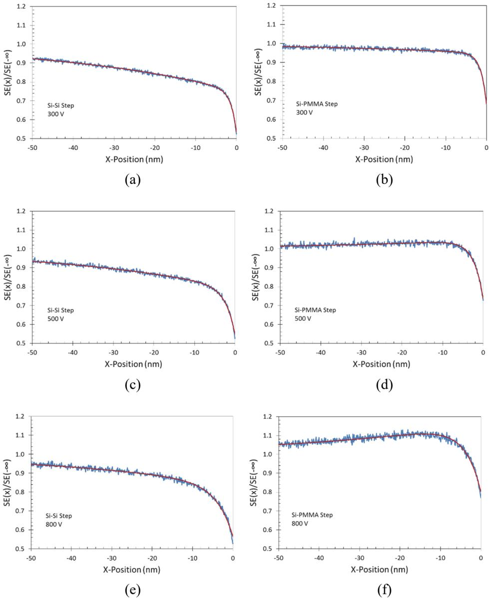
**Figure 4.4** Comparison of Monte Carlo simulations to an analytical model.<sup>17</sup> The smooth (red) line is the equation and the jagged (blue) line is the Monte Carlo simulation results. Both vertical and horizontal comparisons between graphs are enabled by matching the x-axis and y-axis scales of every graph. Note that in this case redundant axes labels could be removed.
