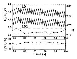
**Fig. 7** Performance of the whole NIR laser diode-based transmittance pulse oximetry system at different processing stages. <sup>26</sup> In the upper part, the PPG signals corresponding to LD1 and LD2 ( $E_1$  and  $E_2$ , respectively) are represented. The middle and lower parts show the q and oxygen saturation ( $SpO_2$ ) values obtained. The dotted lines indicate the lower and higher values of q in the time interval represented.
