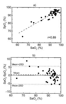
**Fig. 9** (a) Oxygen saturation  $\mathrm{SpO}_2$  values from the NIR pulse oximetry system versus the arterial oxygen saturation obtained from the co-oximeter. (b) The corresponding Bland and Altman plot of the differences with the mean value (mean, dashed line) and two standard deviation values (mean+2 SD and mean-2 SD, dotted lines) between the two sources.
