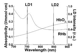
**Fig. 1** Absorption spectra of  $HbO_2$  and  $RHb^{31}$  from 700 to 900 nm and, superimposed, the emission spectra of laser diodes LD1 and LD2. The LD1 emission matches a band of local maximal differential absorption between  $HbO_2$  and RHb spectra. The LD2 emission corresponds to a higher  $HbO_2$  absorption than RHb.
