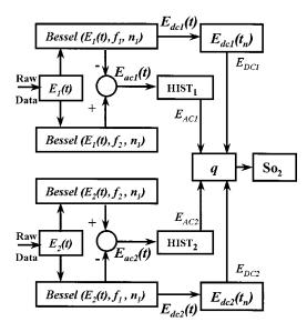
**Fig. 5** Flow diagram of the signal processing algorithm showing the operations performed on both channel signals  $E_1(t)$  and  $E_2(t)$ , Besseltype low-pass filters [Bessel(E(t), f, n)], histogram reduction filtering (HIST), and the variable  $E_{AC}$  and constant  $E_{DC}$  values for each wavelength required for the determination of q and  $SO_2$ .
