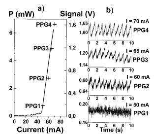
**Fig. 2** The sensor system at different emitter injection current levels in the measurement of a human pulsating vascular bed (distal part of a finger). (a) Continuous-mode power versus current characteristics (–) and the average values (+) of each PPG for the laser diode ILPN-750 in pulsed mode (1  $\mu$ s, 1 kHz). (b) Ten seconds of PPG at different values of injection currents: PPG1 at I=50 mA, PPG2 at I=60 mA, PPG3 at I=65 mA, and PPG4 at I=70 mA.
