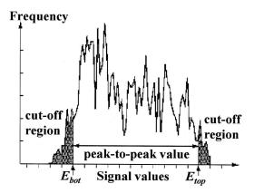
**Fig. 6** Illustration of the histogram reduction procedure. A frequency distribution of the PPG signal values is computed and a fixed sample percentage is rejected from both ends of the distribution (cutoff regions). The peak-to-peak value of the variable component  $E_{AC}$  is calculated from the difference between the maximum or higher value  $E_{\rm top}$  and the minimum or lower value  $E_{\rm bot}$  of the reduced-frequency distribution diagram.
