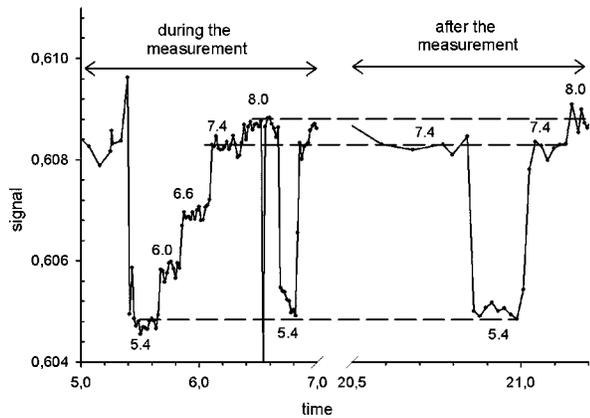
**Fig. 12** Tracing of the pH sensor in the presence of the McIlvaine buffers as carriers in the middle of the *in vivo* measurement and at the end of the measurement; numbers in the tracing indicate the pH values of the McIlvaine buffers flowing through the sensing capillary.
