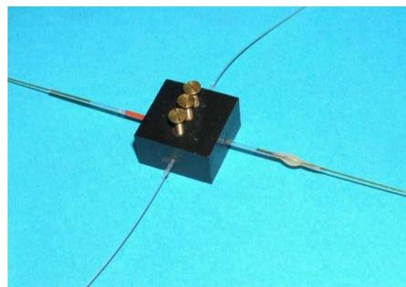
**Fig. 1** Photo of the optical flow cell for the interrogation of the pH-sensing capillary.
