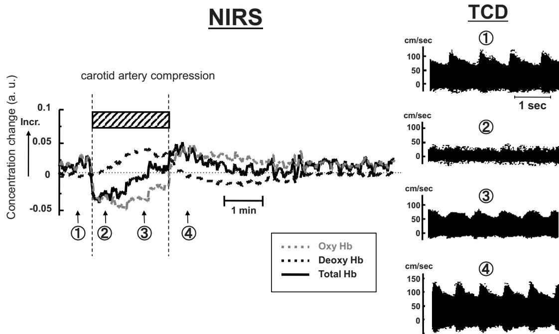
Fig. 1 Changes in cerebral oxygenation and middle cerebral artery blood flow during carotid artery compression. Probes for near-infrared spectroscopy (NIRS) and transcranial Doppler ultrasonography (TCD) were attached on the same side (NIRS numbers correspond to TCD numbers).
