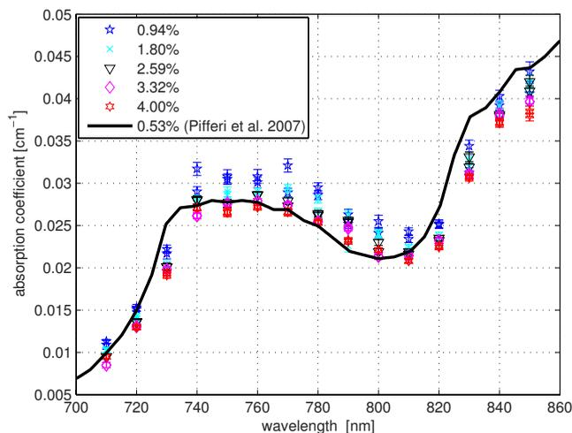
**Fig. 4** Absorption coefficient of Intralipid. Data reported by Pifferi et al.<sup>21</sup> (solid line) are included for comparison. The error bars indicate a 95% confidence interval.
