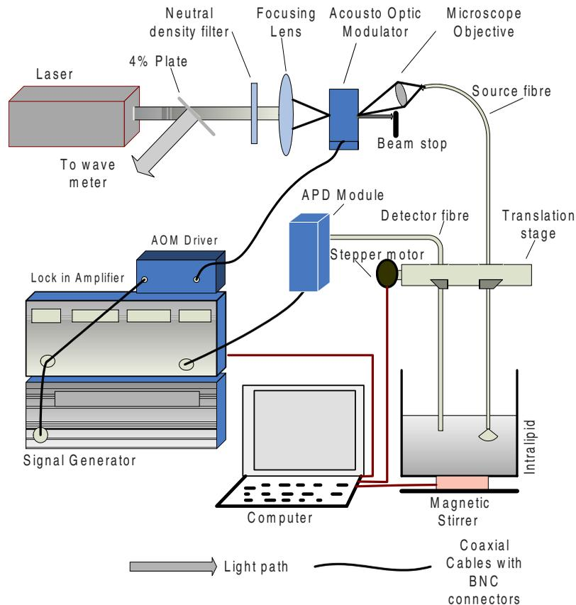
Fig. 1 Schematic diagram of the experiment setup.
