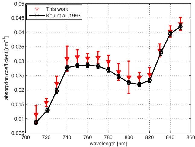
**Fig. 7** Extrapolated absorption coefficient (triangular markers with error bars) for water from Intralipid® measurements versus wavelength. The solid curve represents water absorption data reported by Kou et al.<sup>28</sup> The error bars correspond to  $\pm 2$  standard deviations.
