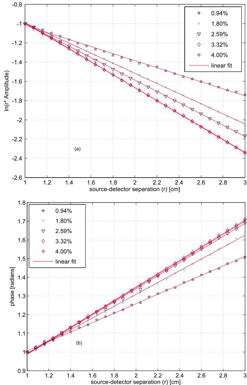
**Fig. 2** (a) Logarithm of source-detector separation times normalized at amplitude and (b) normalized phase variation versus source-detector separation at 750 nm for five Intralipid® concentrations.
