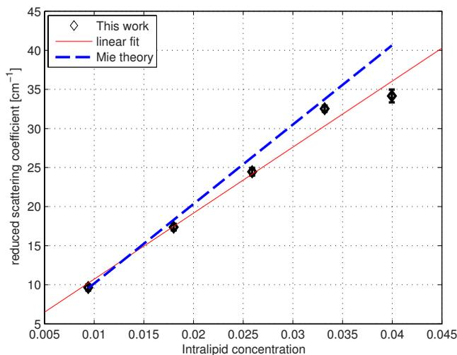
**Fig. 8** Reduced scattering coefficients at 750 nm versus Intralipid® concentration. The errorbars indicate 95% confidence intervals. The solid line is a linear fit to the experimental data. The dashed line shows the Mie theory results.
