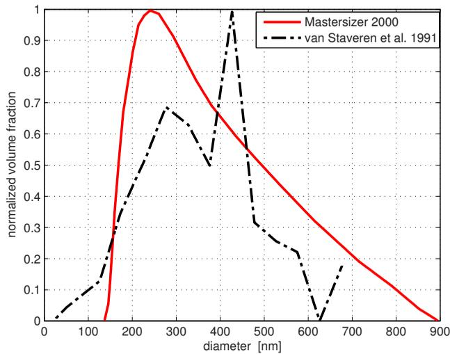
**Fig. 3** Volume fraction of Intralipid@-20% particles measured with a Mastersizer 2000. This distribution is used in our Mie theory calculations. Data by van Staveren et al.,<sup>19</sup> converted to volume fraction, are included for comparison.
