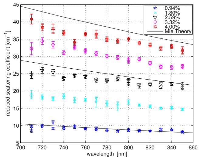
**Fig. 5** Reduced scattering coefficient of Intralipid@. The solid line corresponds to a Mie theory calculation based on our particle-size measurements. The error bars indicate a 95% confidence interval.
