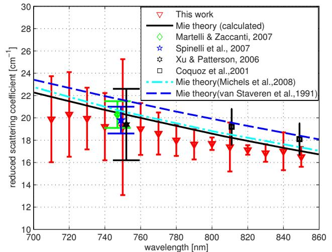
**Fig. 9** Reduced scattering coefficient (triangular markers with error bars) values for a 2% solution of Intralipid® plotted against wavelength. The solid line corresponds to the Mie theory values calculated based on our particle size measurement. Data reported at 750 nm are staggered a little to make them visible. The error bars indicate 95% confidence interval.
