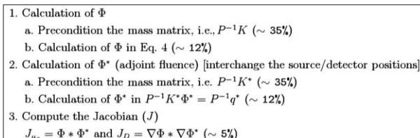
**Fig. 2** Flowchart showing the important computations for calculation of the Jacobian ( $J$ ). The computation time in terms of percentage of total time taken in calculation of  $J$  at each step is also indicated. Note that the calculation of  $J$  accounts for 75% of the total time taken in completing one iteration of diffuse optical image reconstruction (also indicated in Fig. 1).
