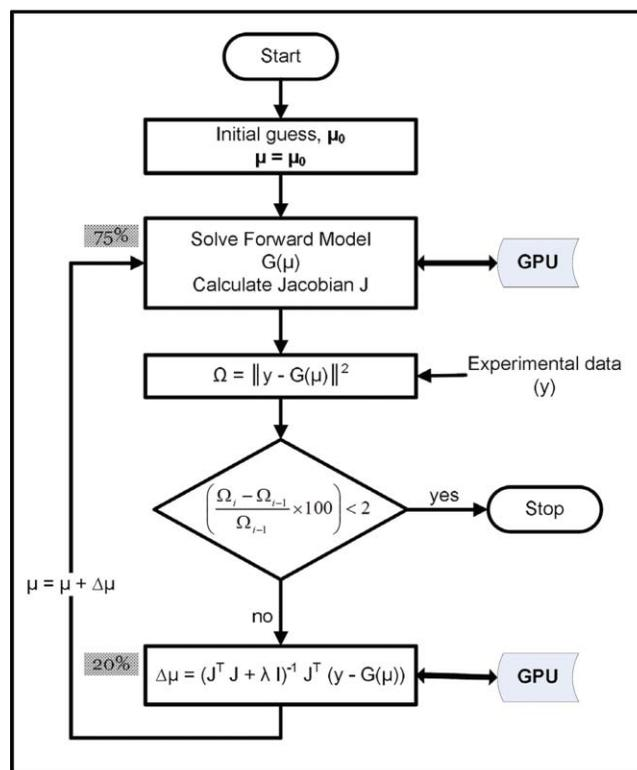
**Fig. 1** Flowchart presenting the important steps involved in reconstructing optical properties in diffuse optical tomography along with associated computation time (in percent of total time per iteration). The steps that used GPU-based computations are indicated with a double arrow.
