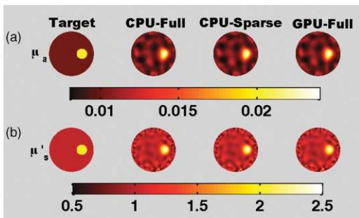
**Fig. 4** Two-dimensional reconstruction results obtained with 1% noisy data using three strategies—CPU-Full, CPU-Sparse, and GPU-Full—discussed in this work. The target 2-D distribution is given in column 1 for (a)  $\mu_a$  images and (b)  $\mu'_s$  images. The number of nodes along with computational time taken for each strategy in a given iteration is given in Table 4.
