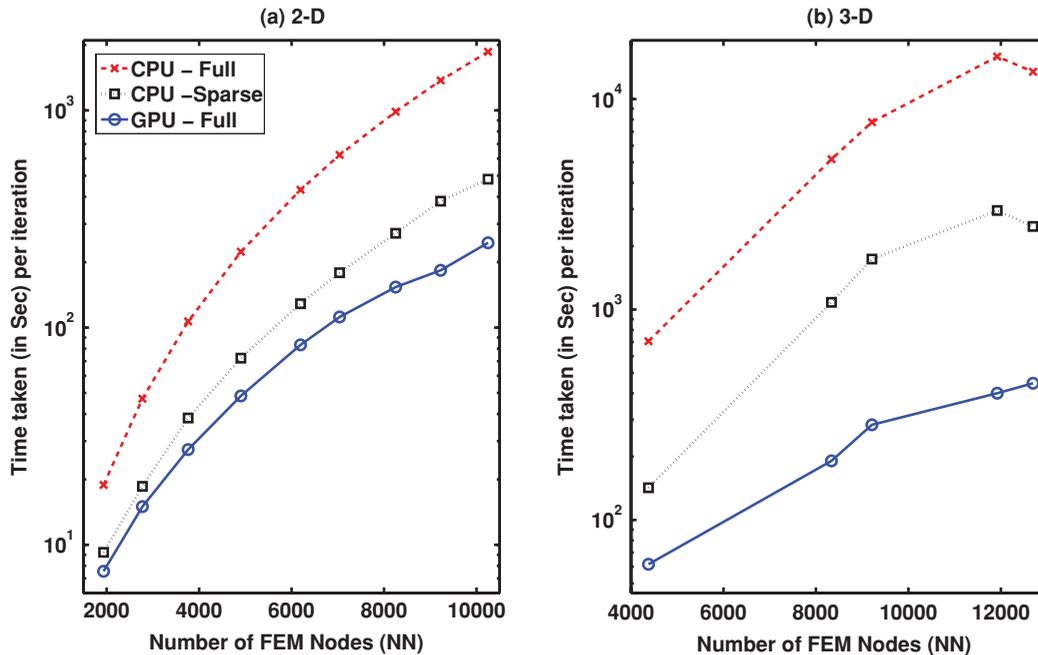
Fig. 5 Plots showing the computation time taken for each strategy [indicated in the legend of (a)] per single iteration versus mesh size (node number,  $N_N$ ) for (a) the 2-D case and (b) 3-D case. The strategies are explained at the end of Section 2.3. The specifications of CPU and GPU are given in Table 2.
