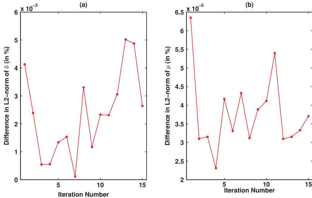
**Fig. 3** Difference (in percent) in the L2 norm between the single- and double-precision computation over the iterations in (a) data-model misfit ( $\delta$ ) and (b) estimated optical properties ( $\mu$ ).
