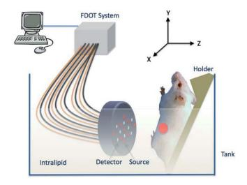
**Fig. 4** *In vivo* fluorescence tomography imaging setup. The live mouse was submerged in 0.6% intralipid scattering medium.
