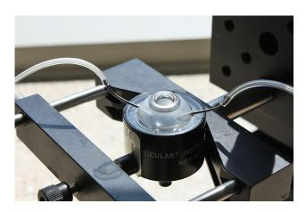
**Fig. 3** Photograph of the custom-built ocular model. Note that the chamber is fitted with two infusion tubes, which allows changing of glucose concentration in the anterior section.
