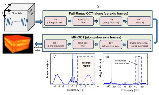
**Fig. 5** Full-range volumetric MM-OCT. (a) Processing steps. (b) Lateral Fourier transform of the fast-axis frame showing the shift in frequency due to the linear-phase modulation along the fast axis. The high-lighted region corresponds to the filtered region. (c) Lateral Fourier transform of the phase differences along the slow axis showing the peak corresponding to the magnetic modulation frequency. The high-lighted region corresponds to the band-pass filter bandwidth.
