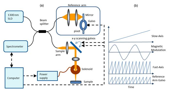
**Fig. 2** Spectral-domain full-range volumetric MM-OCT. (a) Experimental setup. The beam is incident on the mirror at an offset from the galvo pivot in the reference arm, providing the phase modulation along the fast axis for full-range imaging. The electromagnetic coil in the sample arm is driven by a sinusoidal signal to provide the magnetic modulation. (b) The driving waveforms for full-range volumetric MM-OCT operation.
