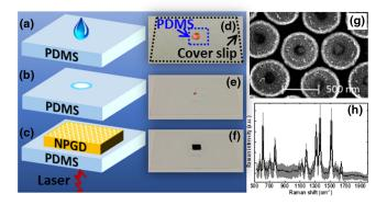
**Fig. 1** Schematics and corresponding images of S-SERS and NPGDs: (a)–(f) See text for details; (g) scanning electron microscopy image of NPGDs; (h) SERS along the laser line from 100  $\mu$ M Rhodamine 6G (R6G) with average spectrum (black solid line) and  $\pm$ 1 standard deviation (gray shade).
