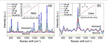
**Fig. 2** Before ("Normal") and after stamping ("Stamped") SERS for: (a) R6G and (b) urea. Insets show (a) R6G peak intensity at 1366 cm<sup>-1</sup> and (b) urea peak intensity at 1001 cm<sup>-1</sup> versus concentrations.
