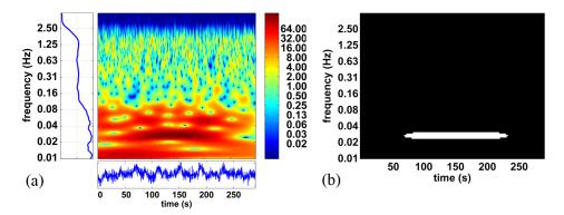
**Fig. 2** Wavelet transform of the channel 17 in (a) and the mask shown in (b). The upper left line plot in (a) presents the power spectral density of the response; the lower right line plot is the channel 17 data in the time domain; and the upper right color map is the scalogram of the wavelet transform of the channel.
