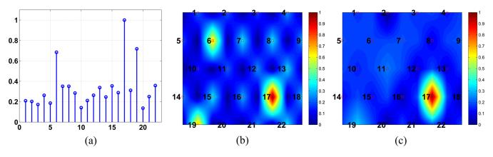
Fig. 5 Normalized coherence of the channels (a) and the activation map in (b) and (c) by the method and GLM method, respectively.
