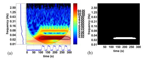
**Fig. 7** Wavelet scalogram of an ideal response in (a) and the mask with significant power in (b). The wavelet transform spectrum in the time-frequency domain is shown in the upper right subfigure of (a). The scalogram in terms of the frequency is shown in the upper left subfigure. The bottom graph shows the predicted response.
