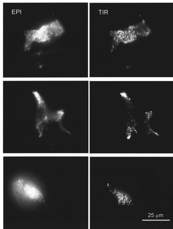
**Fig. 4** EPI vs TIR prismless fluorescence photographs with the Olympus 1.45 NA 60X objective and an argon laser source of wavelength 488 nm. These are three different bovine chromaffin cells containing secretory granules marked with GFP-ANP. The EPI is produced by moving lens L (in Figure 1) in the  $y$  direction until the angle of incidence becomes subcritical. The images were recorded by a cooled monochrome charge coupled device (CCD) camera (Photometrics Star-1).
