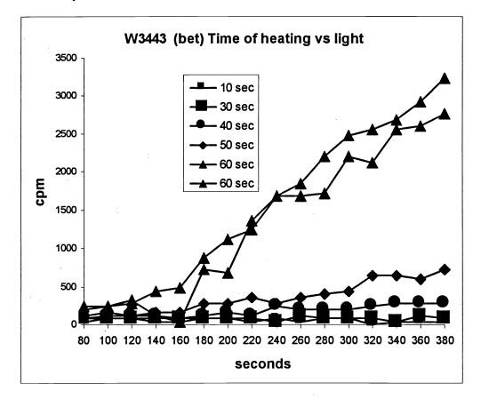
Figure 3. Light emission as a function of the time of heating.
