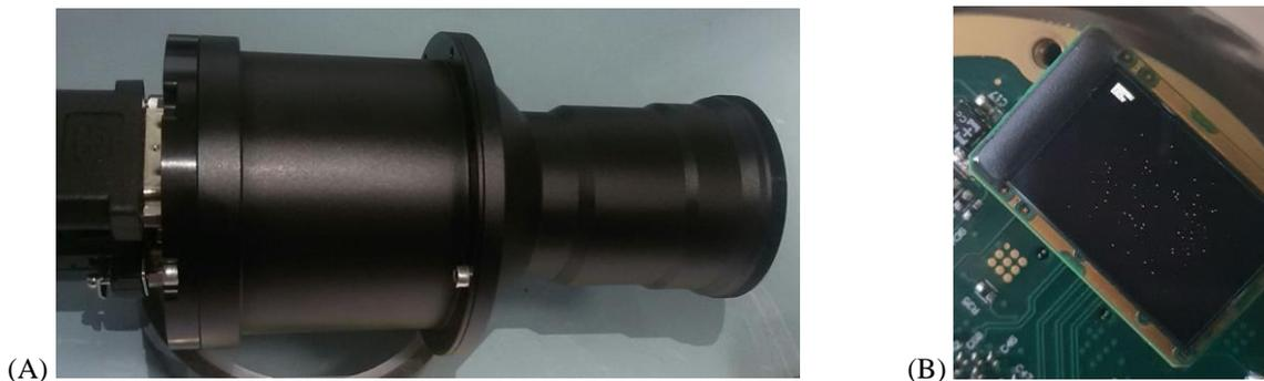
Figure 2. The MINISTAR: (A) the assembled prototype, and (B) the monitor with the rendered star field.
