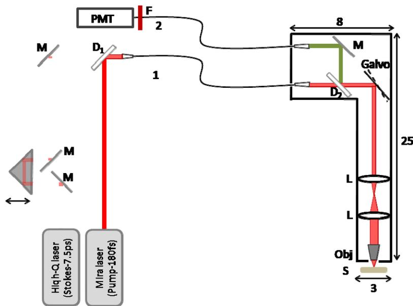
**Figure 2.** Schematic diagram of the fiber-delivered probe for CARS tissue imaging: M- mirrors; D<sub>1</sub>- 1000 nm longpass dichroic mirror; D<sub>2</sub>- 760 nm longpass dichroic mirrors, L- lens; Obj-objective; S-sample; F- 670 nm bandpass filter. Fiber 1 is used for delivery of the excitation pulses and fiber 2 is used for detecting the CARS radiation. The dimensions of the probe are indicated in cm.
