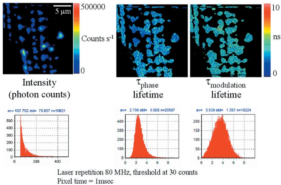
**Fig. 7** Time-domain FLI images of YGFP in *C. elegans* PAT4 construct. The tau phase and tau mod images were calculated using the formulas in the text and if the intensity value was above 30 counts in the pixel.
