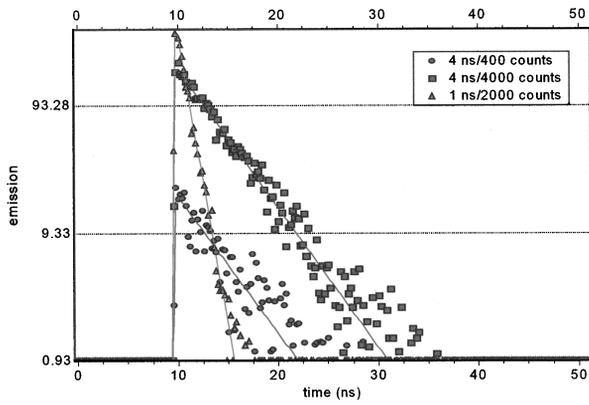
**Fig. 1** Simulated time-domain decay for 4-ns component (4000 counts), 4-ns component (400 counts), and a reference compound of 1 ns (2000 counts). The solid lines correspond to a fit using Globals WE software. The recovered lifetimes are reported in the text. The lamp curve (not shown) has a width of 300 ps.
