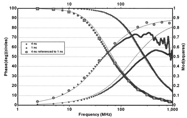
**Fig. 2** Frequency-domain representation after fast Fourier transformation of the data from Fig. 1 of the 4-ns component (4000 counts), the 1-ns component (2000 counts), and the 4-ns components referenced to the 1-ns component.
