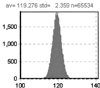
Fig. 6 Phase standard deviation from the time-domain data of an image (256 $\times$ 256) for a 1- $\mu$ M fluorescein solution. The absolute phase value has not been referenced to the reference compound.
