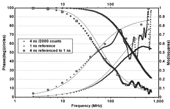
**Fig. 3** Frequency-domain representation after fast Fourier transformation of the data from Fig. 1 of the 4-ns component (400 counts), the 1-ns component (2000 counts), and the 4-ns components referenced to the 1-ns component.
