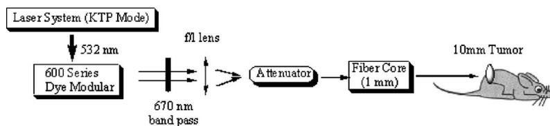
Fig. 1 PDT laser setup for evaluating Pyro-2DG in 9L glioma bearing rat.
