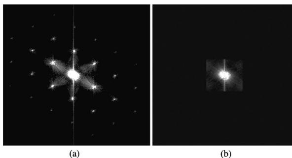
**Fig. 3** (a) The Fourier transform magnitude of the image depicted in Fig. 2(a) clearly showing the periodic noise of the underlying grid pattern. The periodic noise from the bronchoscope fibers corresponds with the bright regions surrounding the center mass. (b) The resulting low pass filtered image in the frequency domain.
