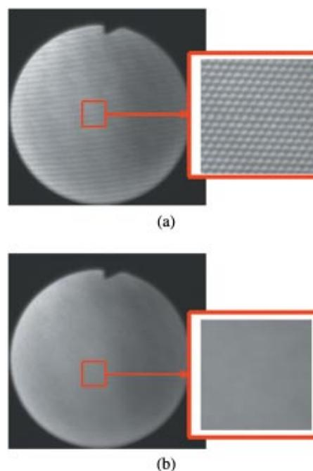
**Fig. 2** (a) White light image captured using the fluorescent imaging system highlighting the underlying fiber distortion and (b) the image postapplication of the Fourier domain filtering.
