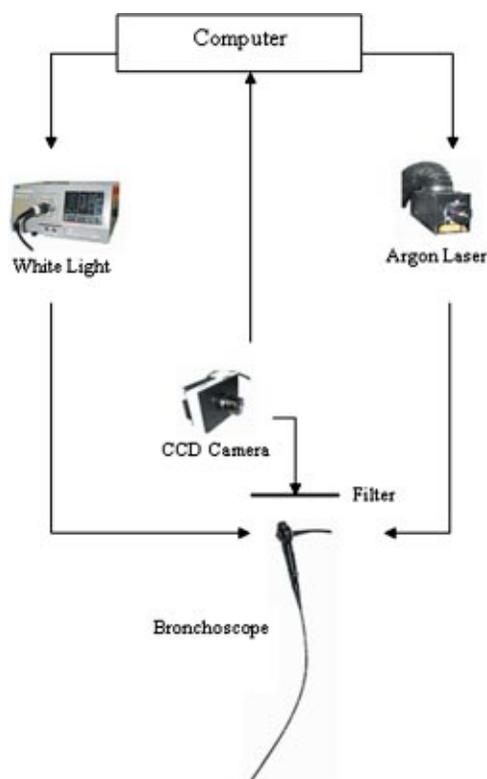
**Fig. 1** Flow diagram of the fluorescent imaging system for use in the detection of green fluorescent protein in the pulmonary airways. The bronchoscope is used to visualize the airways in conjunction with the white light and argon laser. The CCD camera captures images as seen by the bronchoscope with the laser light removed. The personal computer (PC) controls the entire system operation.
