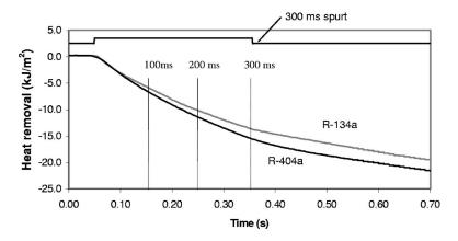
Fig. 3 Comparison of CSC-induced heat removal from the skin phantom in response to R-404a and R-134a spurts: (a)  $\tau_{CSC}$ =100 ms, (b)  $\tau_{CSC}$ =200 ms, (c)  $\tau_{CSC}$ =300 ms.
