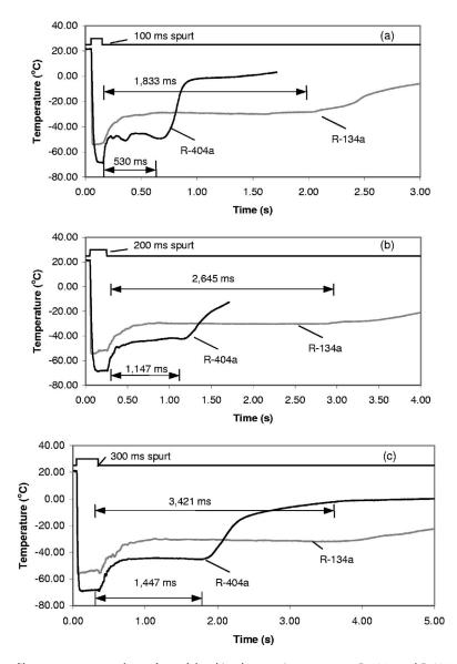
Fig. 1 Comparison of cryogen film temperature on the surface of the skin phantom in response to R-404a and R-134a spurts: (a)  $\tau_{CSC}$ =100 ms, (b)  $\tau_{CSC}$ =200 ms, (c)  $\tau_{CSC}$ =300 ms.
