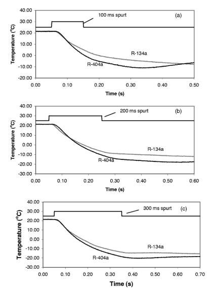
Fig. 2 Comparison of internal temperature at the depth of 100  $\mu$ m below the surface of the skin phantom in response to R-404a and R-134a spurts: (a)  $\tau_{CSC}=100$  ms, (b)  $\tau_{CSC}=200$  ms, (c)  $\tau_{CSC}=300$  ms.
