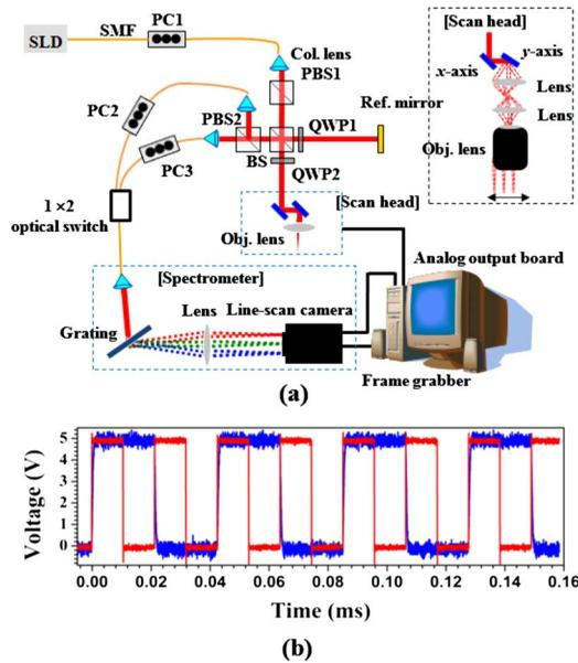
**Fig. 1** (a) Schematic of our PS-OCT system using a single spectrometer and a  $1 \times 2$  optical switch. (b) Timing diagrams to synchronize the line-scan camera with the optical switch. The synchronized line trigger (red) for the line-scan camera with the driving signal for the optical switch (blue). (Color online only.)
