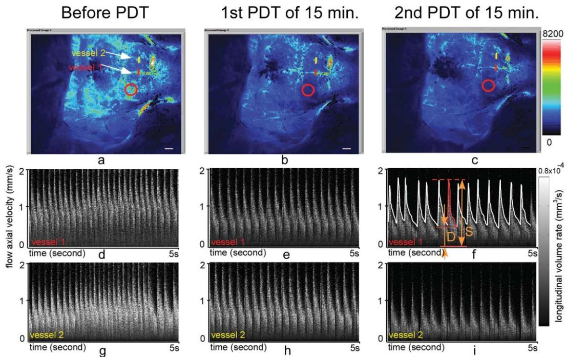
**Fig. 5** Laser speckle flow index maps of the mouse skull (a) before PDT, (b) 15 min after the first PDT, and (c) 15 min after the second PDT, respectively. SDOCTI of vessel 1 [red line in (a)] (d) before PDT, (e) after first PDT of 15 min, and (f) after second PDT of 15 min; SDOCTI of vessel 2 (yellow) (g) before PDT, (h) after first PDT of 15 min, and (i) after second PDT of 15 min, respectively. (All scale bars represent 1 mm.)
