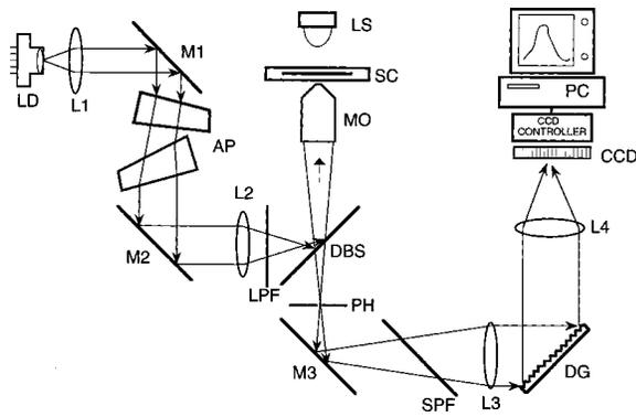
**Fig. 1** Experimental system for implementing optical trap and fluorescence detection. LD: laser diode; AP: anamorphic prism pair; M1–M3: mirrors; L1–L3: lenses; LPF: long pass filter; DBS: dichroic beamsplitter; MO: microscopic objective; SC: sample chamber; LS: light source; PH: pinhole; SPF: short pass filter; DG: diffraction grating; CCD: charge coupled detector; and PC: personal computer.
