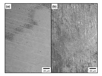
Fig. 6 Zoomed in FESEM images of (a) stainless steel microneedle and (b) agarose microneedle without silver coating.
