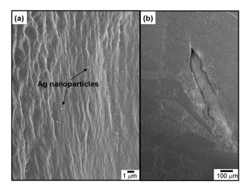
Fig. 9 FESEM (a) image and (b) zoomed-in image of cross-section of phantom after removing the inserted Ag-coated agarose microneedle.
