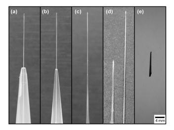
**Fig. 1** Agarose microneedle fabrication steps: (a) agarose in pipette with acupuncture needle, (b) agarose and acupuncture needle removed from pipette, (c) dried for 18 h, (d) agarose microneedle removed from acupuncture needle, and (e) final Ag-coated agarose microneedle. The scale bar is shared by all figures.
