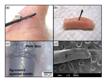
**Fig. 8** Penetration of pig skin at an angle almost (a) parallel and (b) perpendicular. (c) Zoom in image of (a). (d) SEM image of an Ag-coated agarose microneedle with a blunt tip after insertion.
