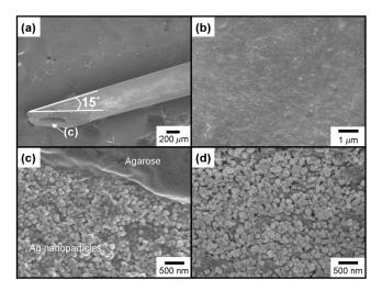
**Fig. 3** Field emission scanning electronic microscope (FESEM) images of (a) Ag-coated agarose microneedle, (b) agarose microneedle without Ag coating, (c) inside the lumen at the tip of the Ag-coated agarose microneedle, and (d) Ag-coated agarose microneedle modified with 1-decanethiol.
