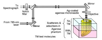
Fig. 2 Schematic of the Raman setup for SERS measurements using a microneedle.
