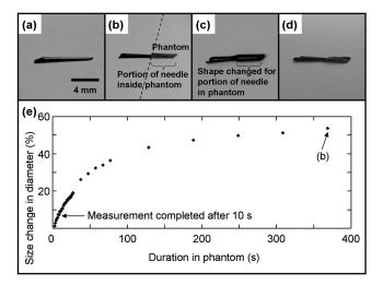
Fig. 7 Ag-coated agarose microneedle (a) before and (b) after insertion into phantom (defined by the dash line) for more than 6 min and (c) removed from phantom after insertion with (d) permanent deformation after pressing onto the tip area. (e) Size variation of agarose microneedle inside phantom as a function of time. At about 10 s, the SERS measurement is completed with a size change of about 9%, in contrast to the variation of 53.9% for another 6 min inside the phantom.
