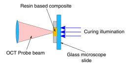
**Fig. 1** Experimental configuration. The resin-based composite was constrained within a 0.75 mm deep, 4 mm diameter ring placed on a glass microscope slide through which the OCT probe beam and the curing lamp illuminated the sample.
