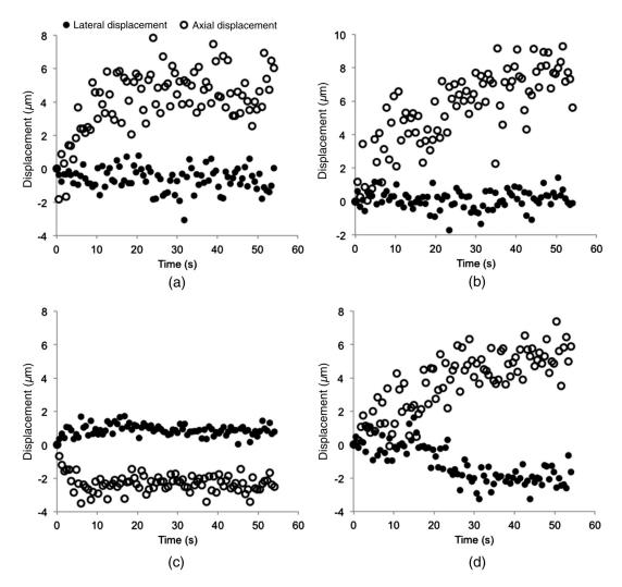
**Fig. 4** Evolution of four displacement vectors (a) to (d), corresponding positions shown in Fig. 3(d) i-iv. The positive axial direction extends from the top to the bottom of the OCT B-Scan and the positive lateral direction is from left to right.
