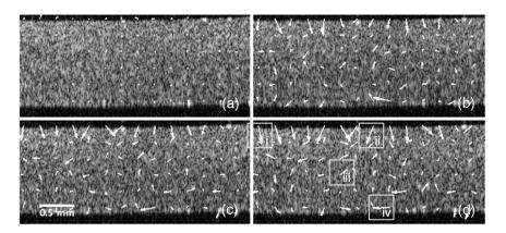
**Fig. 3** Local displacement vectors showing the internal displacement of filler particles at time-points throughout the curing process. (a) Prior to illumination with the curing lamp, t = 0.6 s, (b) at the initiation of cure, t = 3.6 s, (c) t = 5.4 s, and (d) mid-way through the curing process, t = 7.8 s. Boxes i-iv in (d) indicate regions plotted in Fig. 4.
