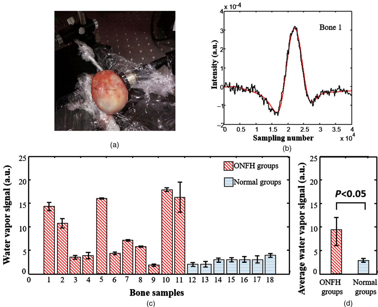
**Fig. 2** The experimental setup and the results for the 18 femoral heads. (a) GASMAS measurement arrangement, (b) water vapor signal from one sample, and (c) data for all 18 samples. ONFH samples are indicated in red whereas normal femoral head samples are indicated in blue. The mean values and SD of the two groups are shown in (d) with a  $p$  value  $< 0.05$ .
