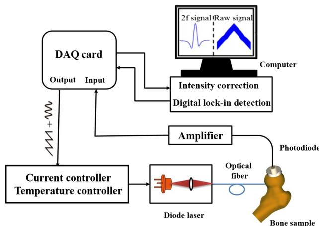
**Fig. 1** The experimental setup for GASMAS measurements of water vapor in pores inside the femoral head.
