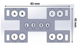
**Fig. 1** Schematic of custom fiberoptic probe with four source positions and eight detector positions. Source positions are denoted 1 through 4, and detector positions are denoted A to H. The corresponding source–detector separations are listed in Table 1.
