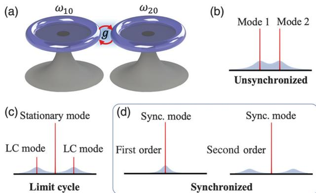
**Fig. 1** Schematic diagram of the system. (a) Two detuned and self-sustained optical microcavities with different resonant frequencies,  $\omega_{10}$  and  $\omega_{20}$ , which are directly coupled at strength  $g$ . (b)–(d) Frequency spectra of the coupled cavities, showing three different long-term states: unsynchronized, limit cycle (LC), and synchronized (Sync.). Light blue represents the noise backgrounds from which the first- and second-order synchronizations are distinguished.
