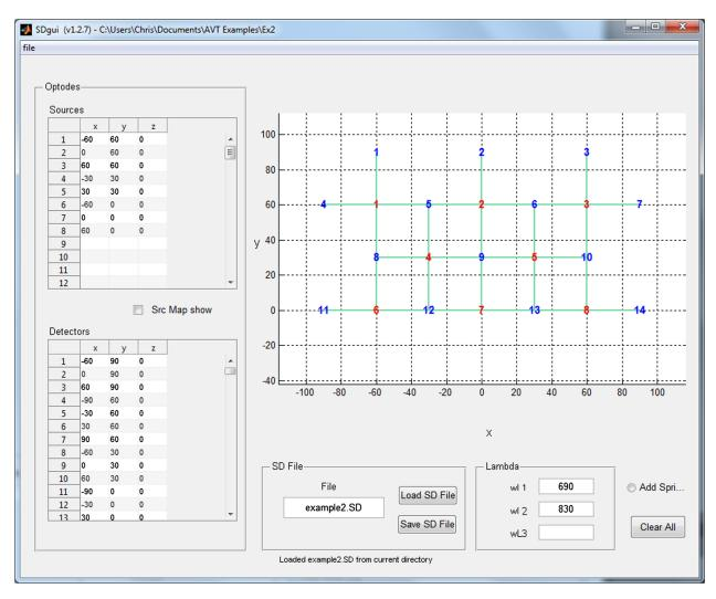
**Fig. 5** This source–detector (SD) configuration provides a laterally symmetrical geometry with sufficient size to encompass the occipital cortex. The alternating SD-source arrangement provides even coverage over a large area.
