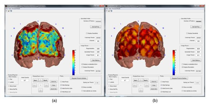
**Fig. 12** (a) The localization error map for the square probe geometry from Sec. 3.1. (b) The resolution map for the same probe. Variation in localization error is highly dependent on the underlying anatomical structure, while probe resolution is predominately a function of source and detector placement. The color scale is linear and spans from 0 to 10 mm as indicated in the "Colormap Thresh" edit box.
