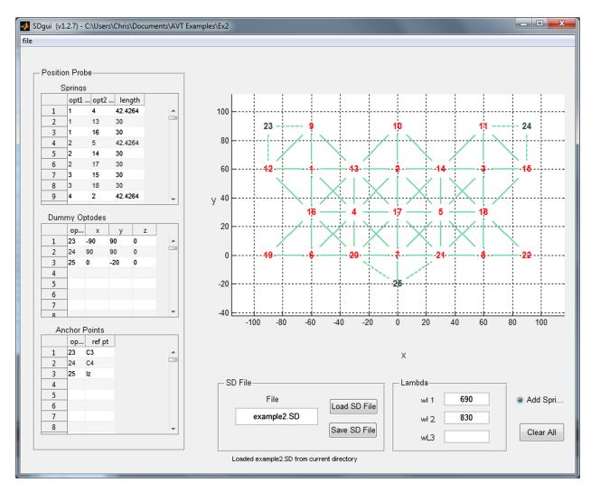
**Fig. 6** The probe in Fig. 5 is intended for the occipital cortex and will need to curve around the rear of the head. To accomplish this, anchor points 23 and 24 are connected to the probe by weak springs and draw the top corners of the probe along the sides of the head while anchor point 25 explicitly holds the bottom of the probe at a specified distance from the inion reference point "Iz" using a rigid spring.
