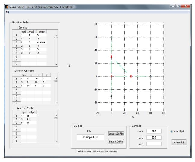
**Fig. 3** The SDgui "Add Springs" window allows the user to create spring connections between optodes, create dummy optodes for the sake of positioning or to reinforce the probe geometry, and to anchor optodes to reference points on the head surface.
