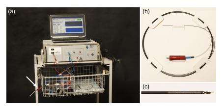
**Fig. 1** Measurement setup. (a) The measurement device with laptop. The white arrow points at the connection point for the fiber. (b) The optical fiber, with a length of 3 m and an outer diameter of 700  $\mu$ m. (c) Incorporation of the optical fiber into 19-G puncture needle.
