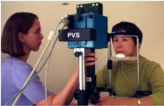
**Fig. 1** Prototype Pediatric Vision Screening device (PVS). The subject is asked to view a blinking target within the aperture of the device. To facilitate testing, the device is mounted on a stand, and the subject's head is placed in a chin rest. Neither the stand nor the chin rest is required for testing. Light emitting diodes (LEDs) indicate passing score.
