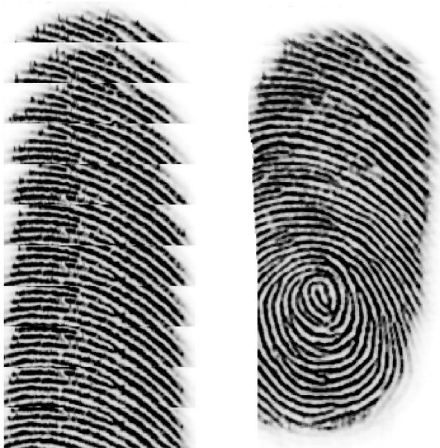
Fig. 2 Fingerprint reconstruction from a sweep sensor: some consecutive frames of a sweep fingerprint sequence and the reconstructed image.
