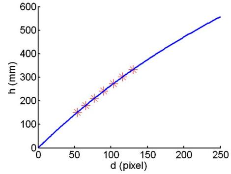
**Fig. 3** Example of the relation between the image lateral shift  $d$  obtained by calibration and the object height  $h$ . Stars present the data collected in calibration.
