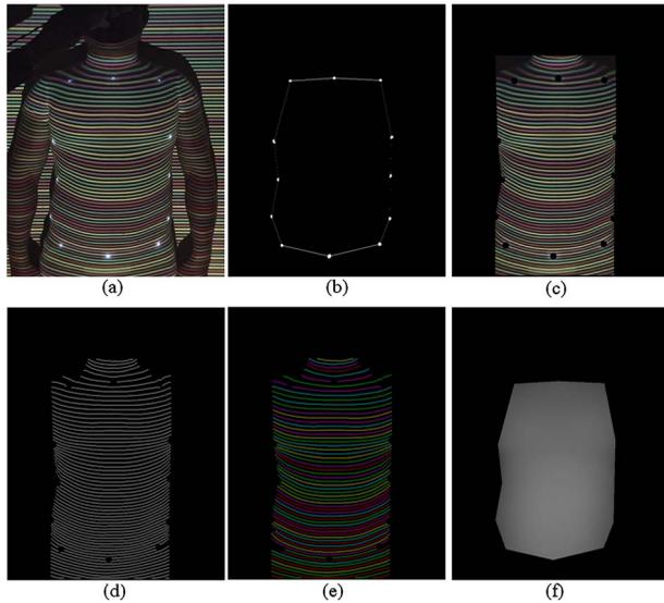
**Fig. 4** Image processing (a) the pattern captured in measurement, (b) the region automatically determined by the segmented markers, (c) the cropped image, (d) the center locations of each color stripe, (e) the recognized color for each stripe, and (f) the calculated depth map. (Color online only.)
