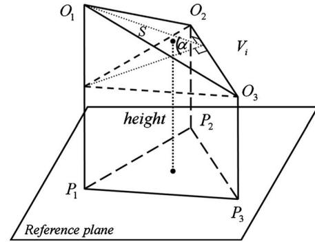
**Fig. 5** Illustration of one column ( $V_i$ ) between a triangle ( $\Delta O_1 O_2 O_3$ ) on the topographic mesh and its projection ( $\Delta P_1 P_2 P_3$ ) on the reference plane: *height* is the distance between the centroid of  $\Delta O_1 O_2 O_3$  and  $\Delta P_1 P_2 P_3$ ,  $\alpha$  is the angle between  $\Delta O_1 O_2 O_3$  and the reference plane, and  $S$  is the area of  $\Delta O_1 O_2 O_3$ . The volume of this column can be calculated by  $V_i = S \cos(\alpha)(\text{height})$ .
