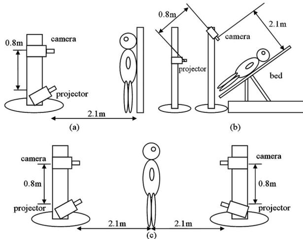
**Fig. 6** Illuminating-recording setups for (a) single-sided standing posture, (b) inclined single-sided supine posture, and (c) double-sided standing posture.
