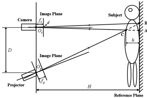
**Fig. 2** Optical geometry of projection and imaging for triangulation measurement.
