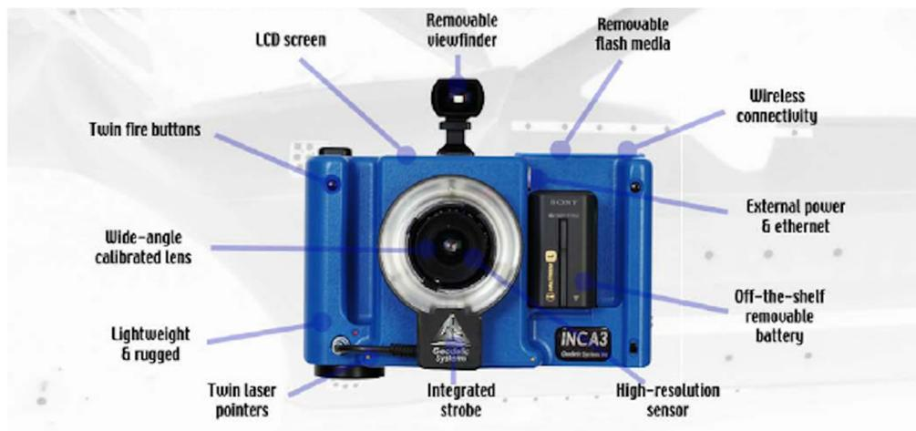
**Fig. 4** INCA3 camera system as provide by GSI.
