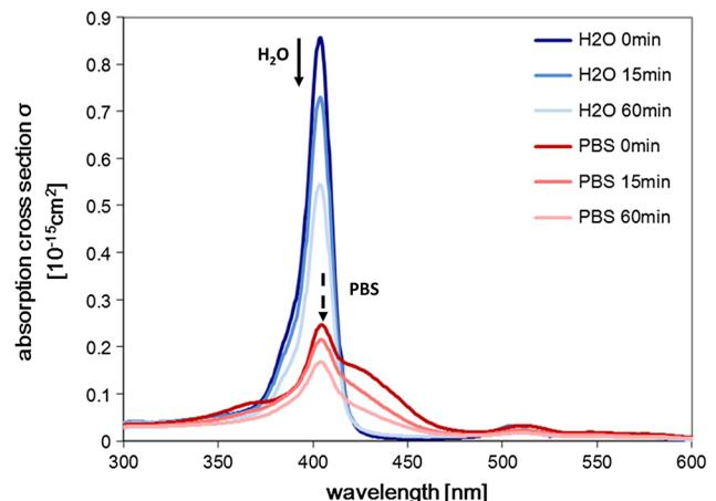
**Fig. 4** Photostability measurements with XF73 show a decrease of the absorption cross section with the time of illumination and therefore the applied energy. The light source was the Waldmann-UV236 lamp with an applied energy dose of  $13.7$  or  $54.7$  J cm<sup>-2</sup>, respectively. XF73 with a concentration of  $10^{-5}$  M has been investigated in pure H<sub>2</sub>O and in PBS (50% in H<sub>2</sub>O).
