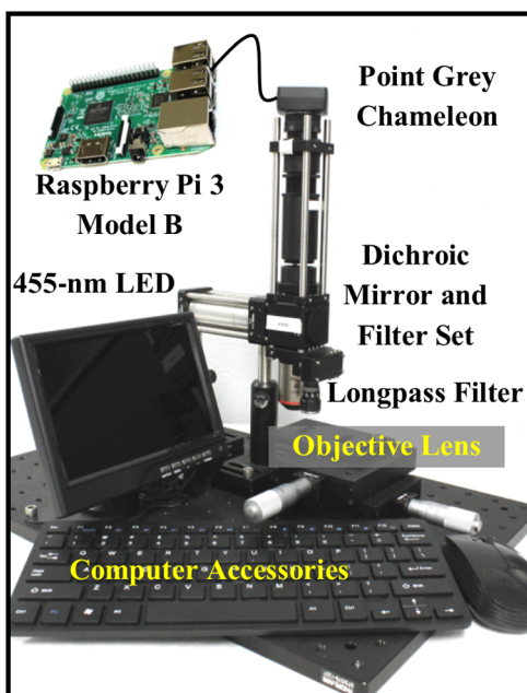
Fig. 2 The imaging system designed to mimic a POC device. It consists of a Raspberry Pi microcomputer connected to an epi-fluorescence microscope with a 4× Nikon Plan Fluor objective, a 500-nm long pass filter, a 475-nm dichroic mirror and filter set, a 455-nm LED, and a Point Grey Chameleon color camera.
