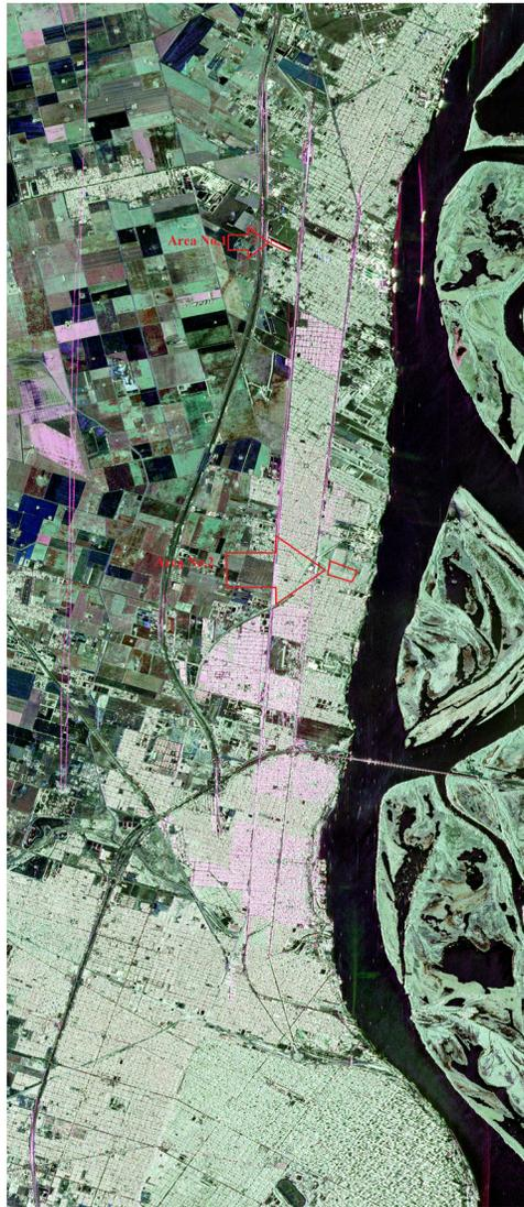
**Fig. 1** The Pauli image of sample data over the area of Rosario, Argentina. This image has been applied a multilook of three looks in range and 12 looks in azimuth. (UAVSAR data courtesy NASA/JPL-Caltech).
