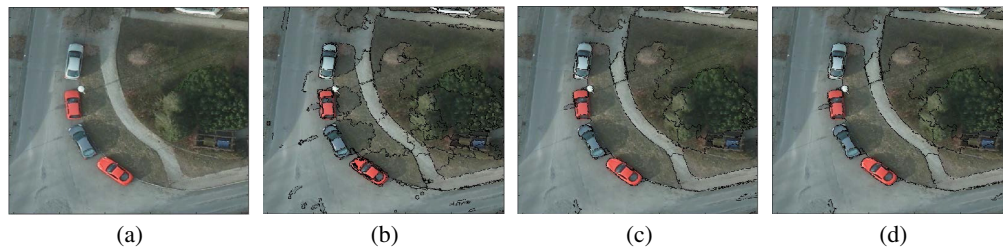
Fig. 7 (a) RGB image patch from Potsdam dataset. (b), (c), and (d) Segmentation results of GSEG algorithm with initial seed size of 15, 100, and 150, respectively.
