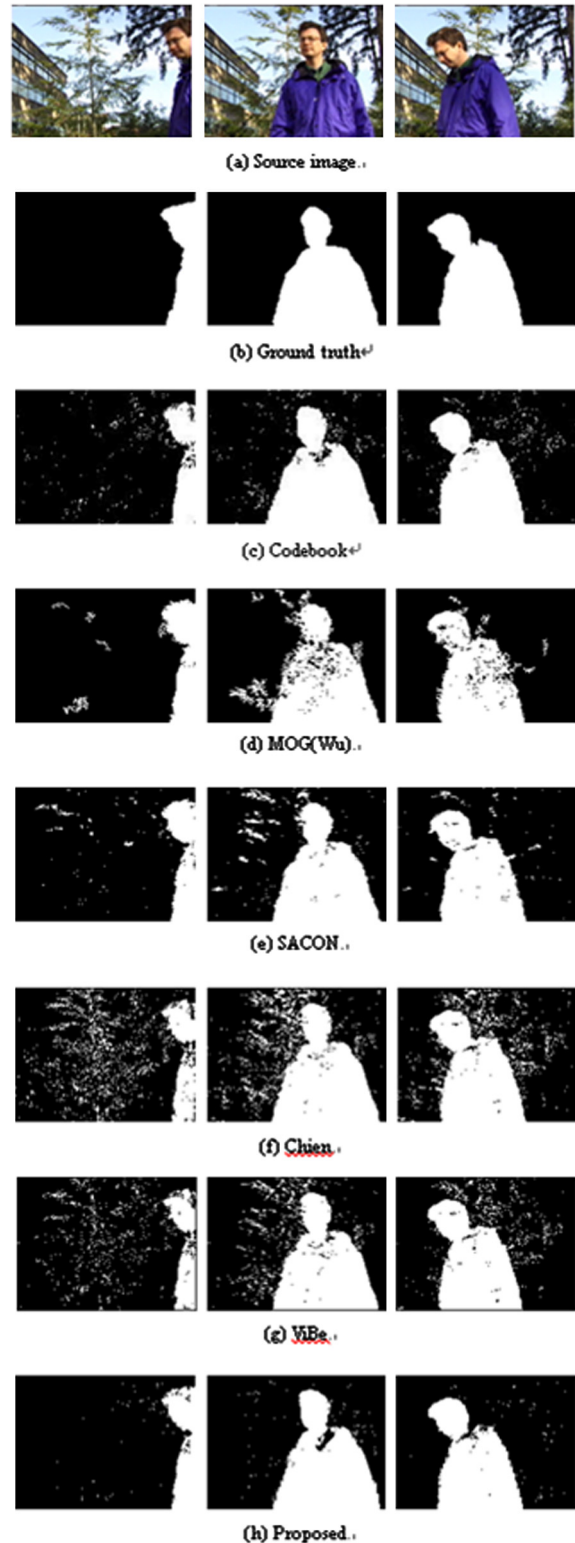
Fig. 5 Object detection results in a moving background: (a) source image, (b) ground truth, (c) Codebook, (d) MoG (Wu), (e) SACON, (f) Chien, (g) ViBe, (h) Proposed.
