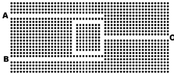
Fig. 20 Structure of OR gate with A and B as input ports.
