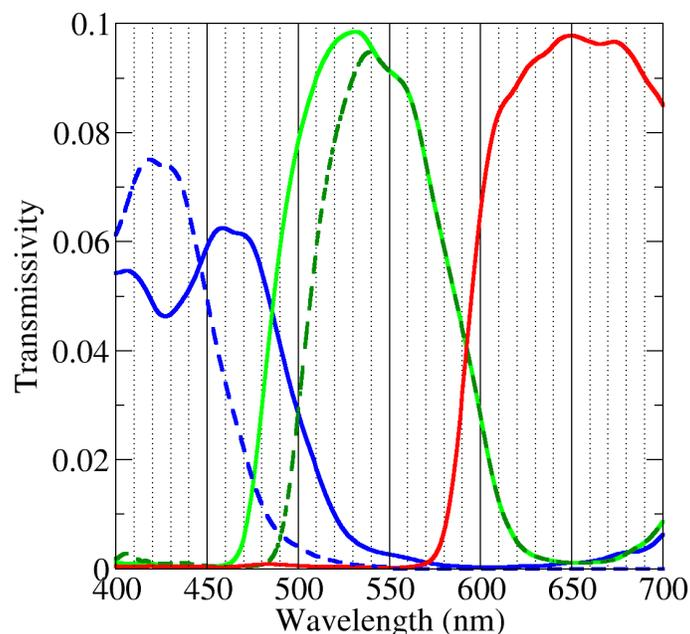
Figure 5: Solid lines: existing color filter transmission coefficients. Dashed lines: proposed color filter transmission coefficients for QD-LCD with Rec.2020 color gamut. The red color filter transmission coefficients are the same.
