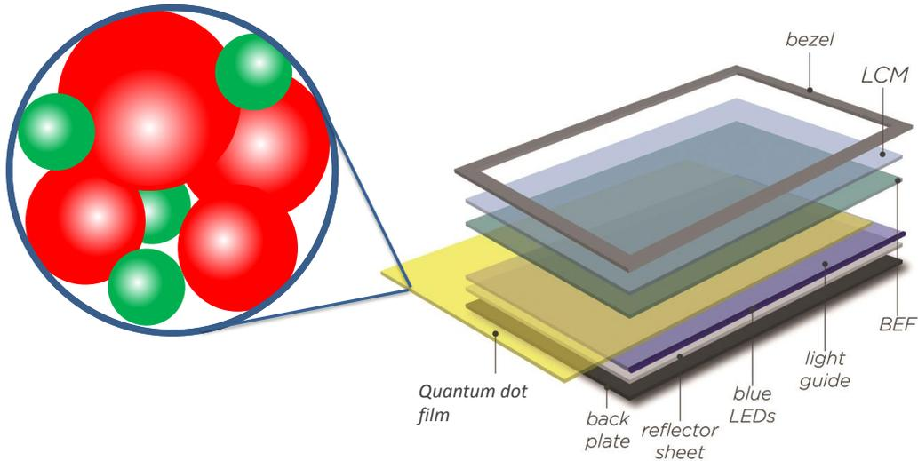
Figure 2: Schematic structure of an edge-lit LCD display with quantum dot film.
