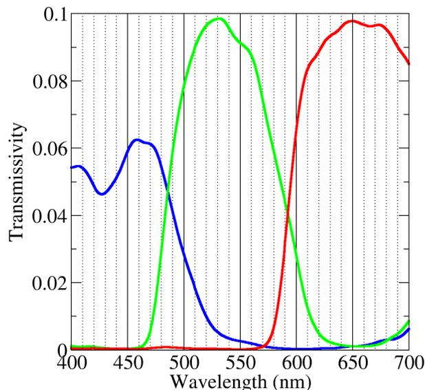
Figure 1: Blue, green, and red color filter transmission coefficients of a typical Rec.709 LCD display.
