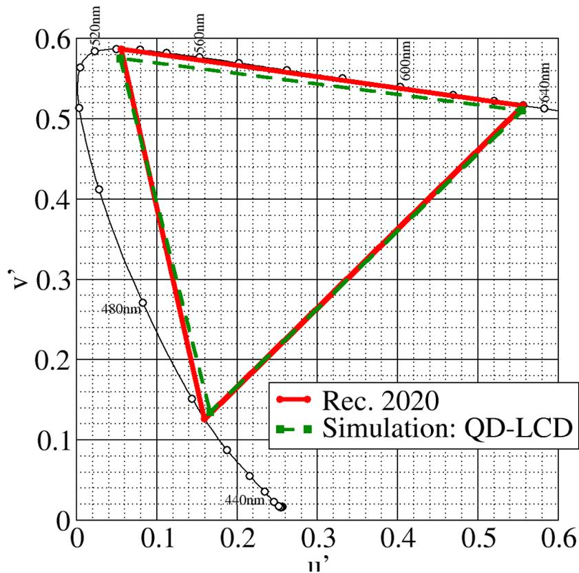
Figure 6: 1976 cie diagram with Rec.2020 and simulated QD-LCD with proposed color filter transmission coefficients plotted in Figure 5. The simulated QD-LCD covers 95% of Rec.2020 color space.
