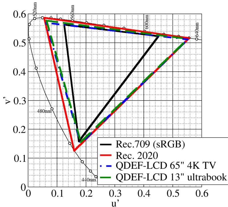
Figure 4: 1976 cie diagram of two LCD demos using quantum dot films, Rec. 709 and Rec. 2020 color standards. The color gamut of both demos covers 90% of Rec. 2020 color space.
