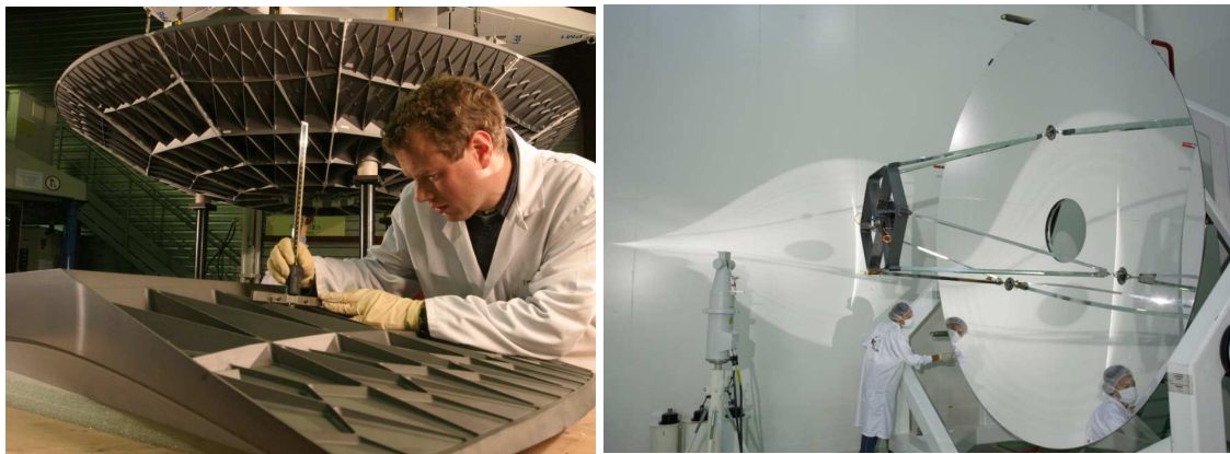
Fig. 2. Herschel a) rear face of brazed primary mirror and b) final telescope assembly
