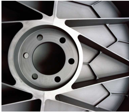
Fig. 3. Detailed view of the rear face of HERSCHEL \Phi 3.5m primary mirror, including an interface
