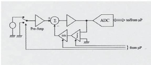
Fig. 4 Simplified block diagram of the sensor channel processing electronics
