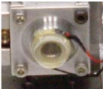
Fig. 1. High stiffness holed piezo actuator (the yellow item where wires are connected to) with the cavity mirror glued on it.
