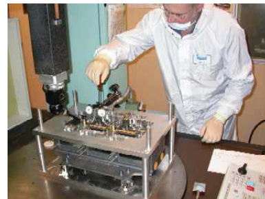
Fig. 8. Assembly of mirrors on the structure on Pleiades EM model
