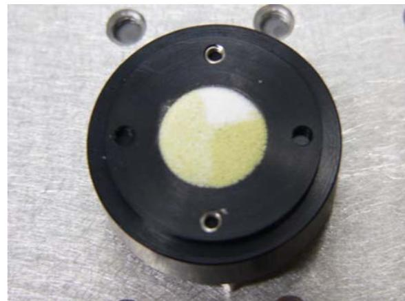
Fig. 5: Image of a sample analysed with MicrOmega. It is composed of three different areas, two made with a pure component (a sulfate and a clay) and a mix of both components
