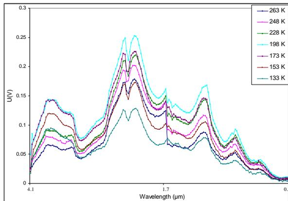
Fig. 10: Thermal test done on a demonstrator AOTF. It shows that we have now a technology that works at low temperature (down to 140 K).
