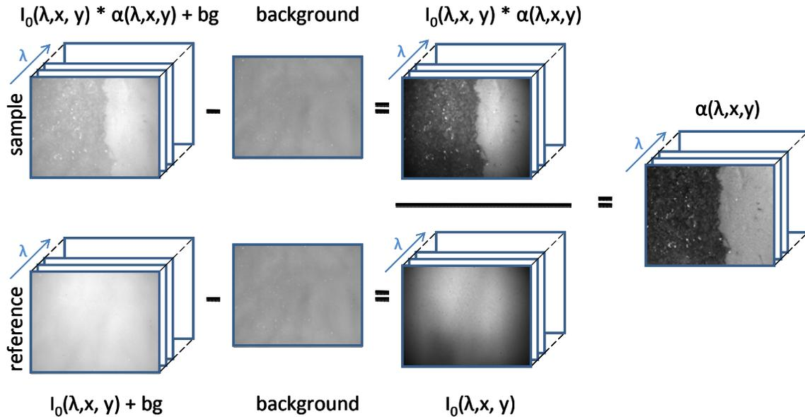
Fig. 4: Protocol used to acquire and measure the reflectance of a sample.
