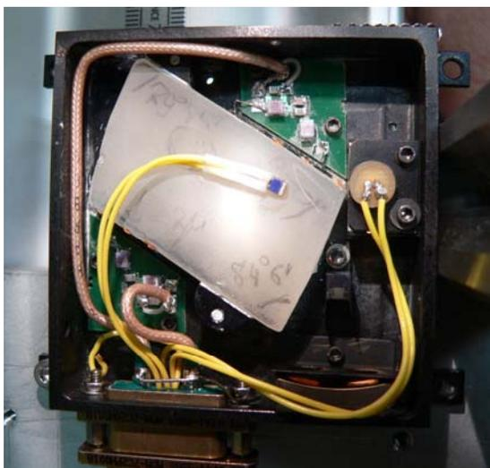
Fig. 2: The AOTF and its illumination system used in the breadboard.
