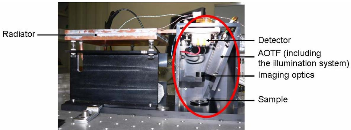
Fig. 1: MicrOmega Breadboard. The demonstrator of the instrument is shown in the red ellipse. The size of this box is 120 mm height and 80 mm width.
