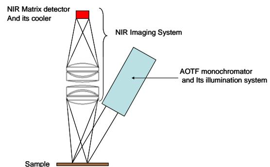
Fig. 3: Optical diagram of the demonstrator of the MicrOmega Instrument. The AOTF output beam makes an angle of  $20^\circ$  with the optical axis of the NIR imaging system
