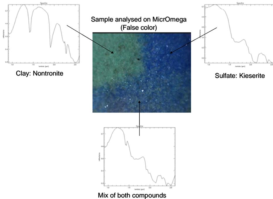
Fig. 6: The same sample as in fig. 5 analysed by the MicrOmega instrument. The image in the center is in false colors. For each area, a spectrum is shown.
