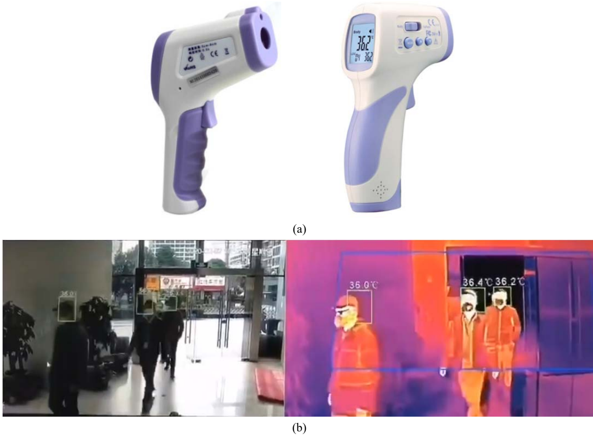
Fig. 1: Body temperature measurement tools: (a) Non-contact Infrared Forehead Thermometer; (b) Crowd temperature monitoring system using both visual and thermal camera .
